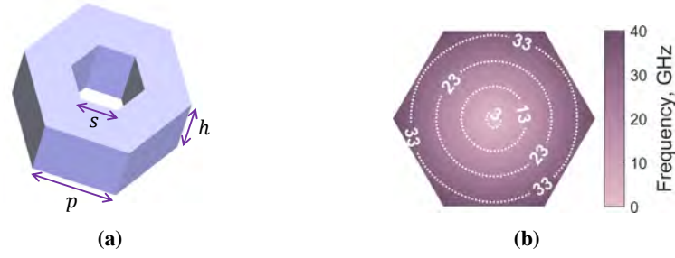
Figure 1. (a) Configuration and design parameters of the 2-D dielectric square unit cell. p and h are the side length and height of the unit cell, and s is the side length of the hexagonal hole located at the center of the unit cell. (b) Isofrequency map (2-D dispersion diagram) of the fundamental mode in the investigated periodic structure. The dimensions of the unit cell used in the simulations are p = 2.0 mm, s = 0.875 mm and h = 2.0 mm. The dielectric material has a relative permittivity of 2.25.
