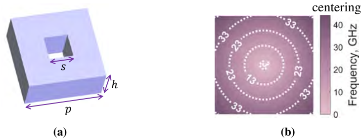
Figure 2. (a) Configuration and design parameters of the 2-D dielectric square unit cell. p and h are the side length and height of the unit cell, and s is the side length of the square hole located at the center of the unit cell. (b) Isofrequency map (2-D dispersion diagram) of the fundamental mode in the investigated periodic structure. The dimensions of the unit cell used in the simulations are: p = 3.22 mm, s = 1.41 mm and h = 2.0 mm. The dielectric material has a relative permittivity of 2.25.
